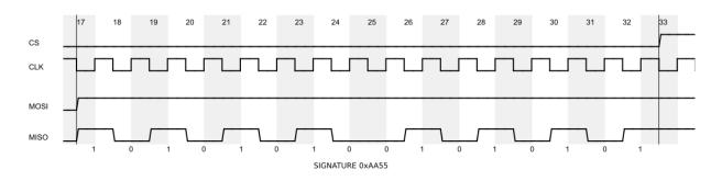
Figure 2: Example - Read SPI\_REG\_SIGNATURE 2/2
