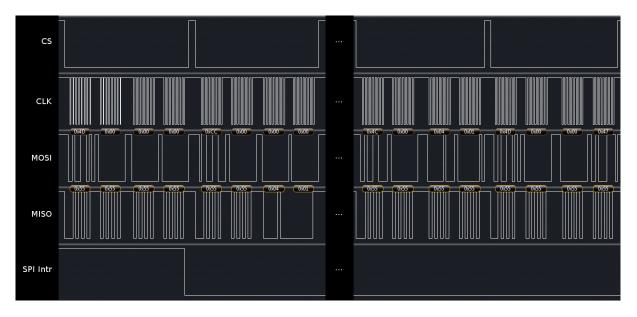
Figure 3: Example - Interrupt handling
